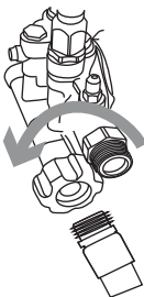
Figure 2-9. Connect Water Supply Hose
