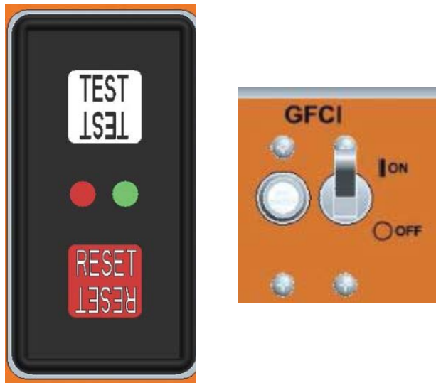
Figure 12 - Testing the GFCI
