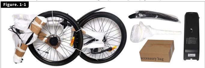
(2) Remove all of the inside cardboard protection and bubble wrap on the bike. Please locate and set aside the kit box containing the battery charger, pedals, and tool kit, etc (Figure. 1-2).
