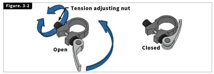
**Please Note**: If necessary, tighten the clamp by twisting the clamp handle clockwise while in the un-clamped position. Then, fold the handle in toward the seat post. This should require a fair amount of force to ensure the seat post is held tight. If necessary, the clamp can be further tightened with a 5 mm Allen wrench while in the clamped position.
