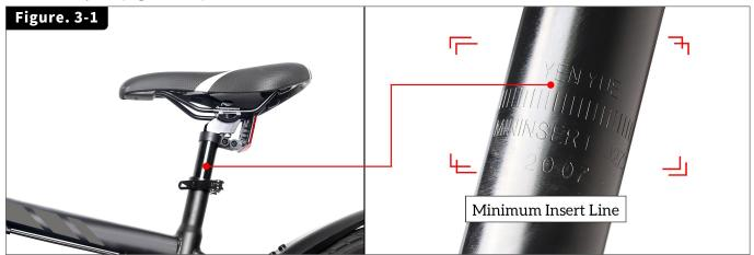
Warning: It could break the seat tube during riding if the seat post does not install correctly. It is not covered by the warranty.
