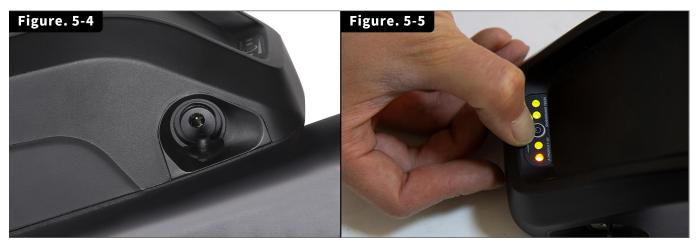
**4. Fuse**: There are two Fuses on the battery. Charging Fuse: 10A, Min. 60Vdc; Discharging Fuse: 30A, Min. 60Vdc. (UL certified Fuse)
