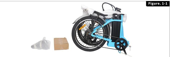
(3) Unfold the bike, Please locate and set aside the kit box containing the battery charger, pedals, and tool kit, etc. (Figure.1-2)
