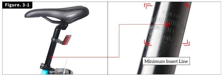
Warning: It could break the seat tube during riding if the seat post does not install correctly. It is not covered by the warranty.
