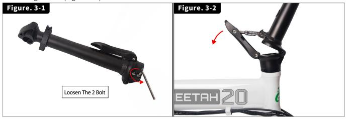
Method: There is a small spherical handle on the side of the handle, pull it to the top, and then pull the handle outward. Fold the stem, and place the plastic cover into it. Tighten the screws (Figure 3-3), then restore the stem to its original state (Figure 3-4).
