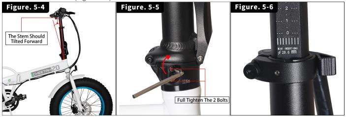
WARNING: It may cause the stem tube to rupture and cause a serious accident if the min insertion line is out of the tube. The customer is responsible for accidents caused by improper installation.
