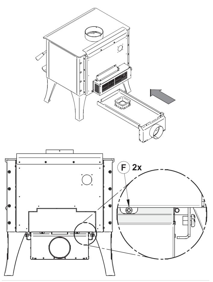
Step 5. Fix the air intake on the front of the stove with two screws  $(\mathbf{F}, 2x)$ .
