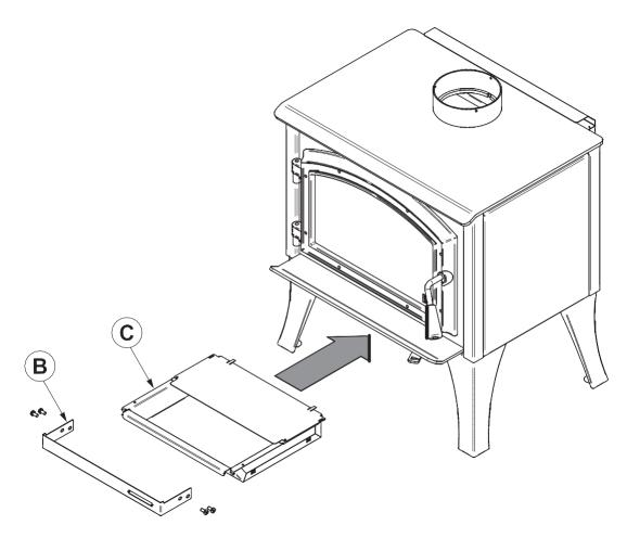
Step 7. Fix the air control cover (B) on the stove using screws (A, 4x) kept from Step 1.
