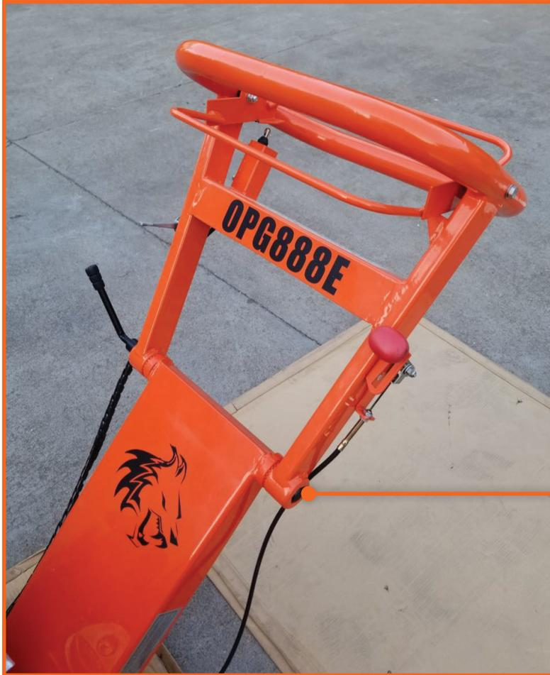
INSTALL THE BOW HANDLE USING THE LONG BOLT AND SPIN HANDLE PROVIDED. ALIGN THE TEETH AND TIGHTEN.
