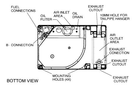
**Note:** This outline drawing is provided for general reference only and is not intended for design or installation. For more information see Operation and Installation manuals or obtain drawing 500-3234 and wiring diagram from your distributor/dealer.
