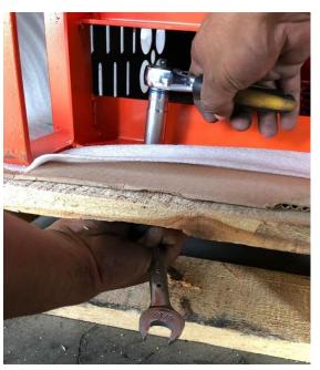
6. Once pallet hardware is removed and using appropriate equipment, safely place the mixer upright on the tires/ground.
