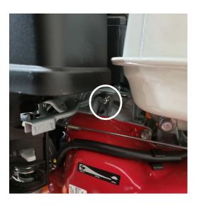
4) Adjust the engine maximum high speed screw, to reach the desired drum rotation speed of 28-30 revolutions per minute, by turning this speed adjustment screw, located on the bracket of the throttle lever, just under the air cleaner cover. Turn left to increase engine RPM, turn right to decrease engine
