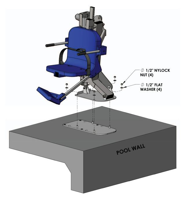
Apply the ANTI-SEIZE lube to the welded stud threads before installing. This will reduce corrosion and prevent the stainless steel from galling.
