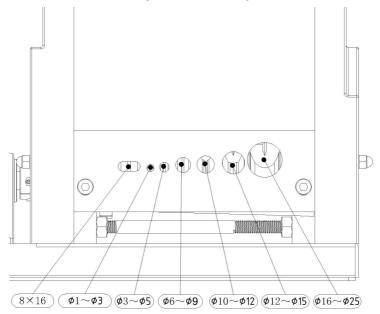
2. During wire stripping, the center of the blade must be collinear with the center of the roller.
