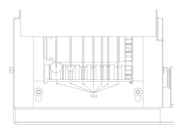
3.According to the thickness of the wire, adjust the distance between blade and rolling shaft so that the blade can cut the wire skin without damaging the copper core ,Adjust the M12 plastic handle screw to adjust the height of the blade through the spring assembly.It would be better to make the blade can cut the wire skin without damaging the copper core.
