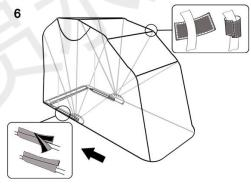
Fold the cover backwards over the frame, wrap the velcros around the ribs as appropriate, and tidy up the whole tent.
