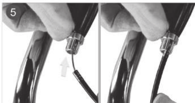
5. Fix the brake cable housing into the brake lever.
