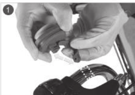
1. The yellow dotted line on the right handlebar is the location where the bell is installed.
