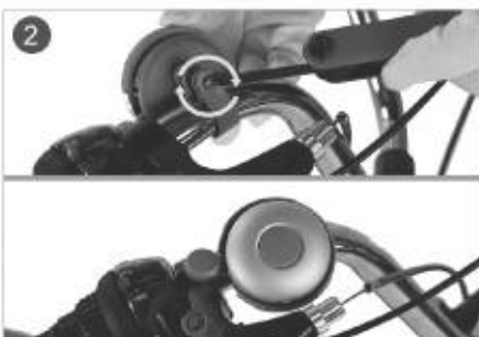
2. Tighten with a Phillips screwdriver
