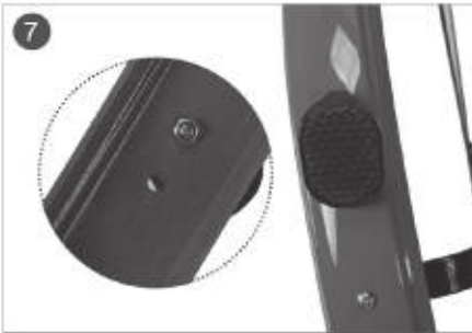
7. Two rear reflectors mounted on the left and right fenders
