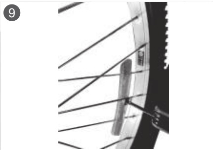
9. Three spoke reflectors mounted on the spokes of two rear wheels and one front wheel
