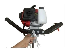
d. Secure the wire and handle with 19# Nylon ties (2pcs) $_{\mbox{\tiny o}}$
