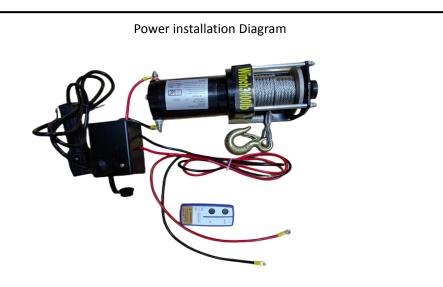
This product is suitable for vehicle, the required input voltage is 12V. Connect the longer end of the wire on the No. 6 fitting (power box) directly to the car power supply, and the shorter end of the wire to the winch end screw. Finally, the wired remote control can be inserted into the power box for use. We also included a wireless remote control for your use.
