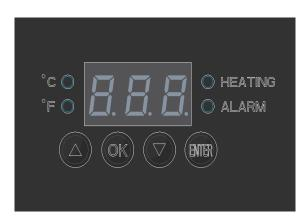
he "" key to adjust the time required for setting transfer. After setting, press the "OK" key again. At this time, the setting is completed and the machine enters the heating state, The temperature control meter displays the real-time temperature.
