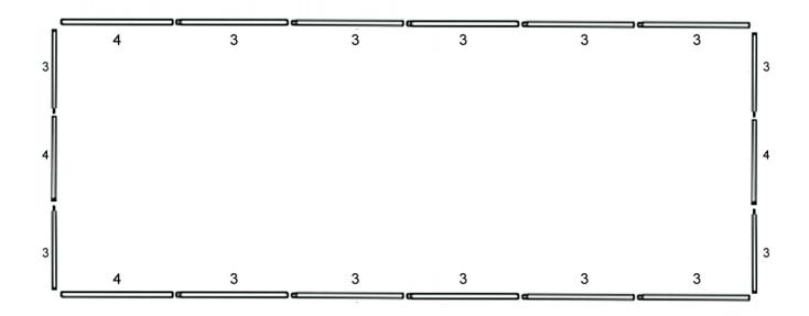
Assemble for 2 sets floor tubes No3+No4+No3 use the shorter bolts, and the horizontal frame No4+No3+No3+No3+No3+No3+No3+Ostogether
