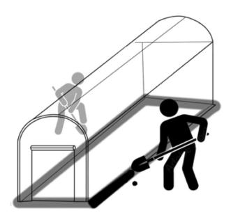
Put the frame inside the trench, ,filling with the soil
