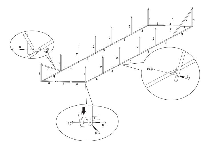
Loosely assemble complete frame, before tightening all bolts in final position.
