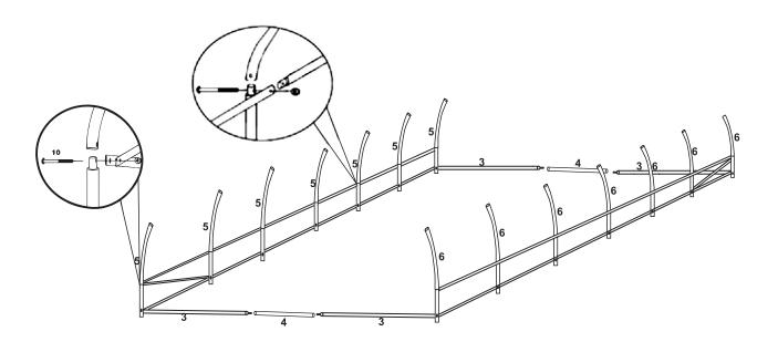
Loosely assemble complete frame, before tightening all bolts in final position.
