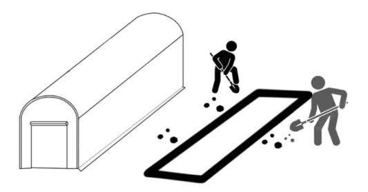
For maximum stability of your polytunnel,we recommend digging a 20cm width trench around the base of the polytunnel and back
