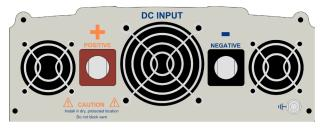
**IMPORTANT:** For 1500 Watt units and less, use a minimum of 2 AWG wire with a wire length not to exceed 4 feet\*.
