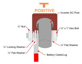
**IMPORTANT:** When fully tightened, the Cable Lug should not be able to rotate around the Inverter connection post. Check and tighten the end caps periodically as they can become loose from vibrations or thermal cycling.
