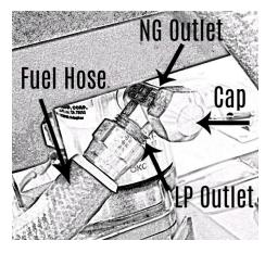
4. Attaching the Propane (LP) or Natural Gas (NG) hose to the generator. Attach the propane or natural gas hose to the male flare fitting on the front of the low pressure regulator using a wrench. Do not over tighten.
