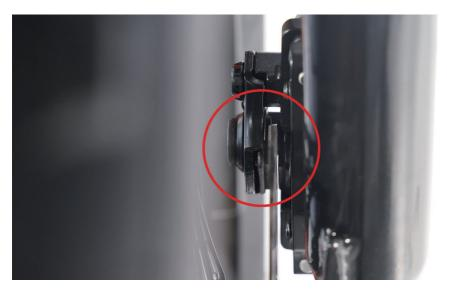
3.Check that the wheel is fully seated in the dropouts and that it is centered. Hold the quick-release lever in line with axle and tighten the thumb nut on the opposite side until the lever can stay parallel to the floor without being held.
