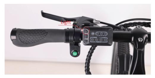
4.Select the desired level of pedal assistance—Select the level from "Low" to "High" by pressing "\[ \times \]" and "\[ \times \]". "Low" corresponds to the lowest level of pedal assistance, and "High" corresponds to the highest level of pedal assistance. Start in PAS level "Low" and adjust from there.
