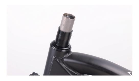
3.Install the handlebars onto the steer stem.
