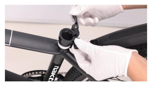
2.Insert seat post into seat tube. Adjust the seat post up or down to a comfortable height, while ensuring the seat post is inserted into the frame past the minimum insertion point.
