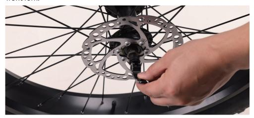
2.While keeping the lever open, lift the front of the bike and lower the fork onto the wheel axle. **Notice:** The brake rotor should go into the brake caliper in between the brake pads and the axle should enter the fork dropouts fully. The front rotor orientation should be to the left of the fork.
