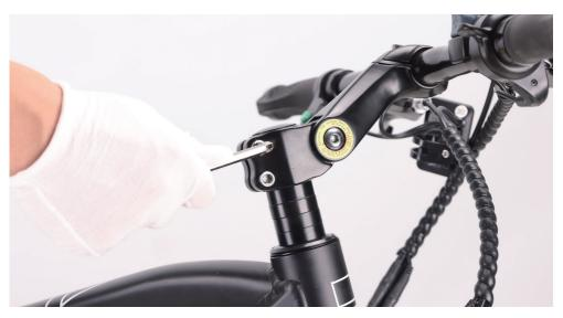
6. Tighten the bolt on the top of the steer stem with the supplied allen wrench.
