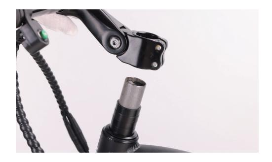
4. Pass the stem bolt through the washer mounting point and the stem mount, tighten with the supplied allen wrench part away.
