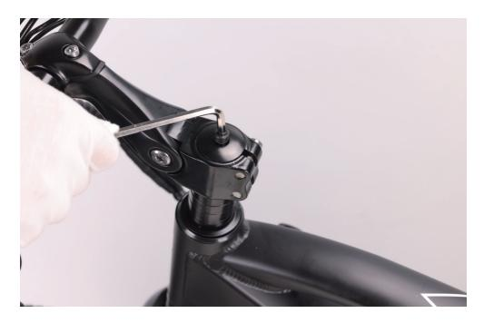
5.Align the stem so the handlebar is perpendicular to the front wheel. Use the allen wrench to tighten the stem clamp bolts evenly (a half turn at a time alternating between the two bolts).
