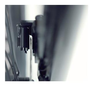
On the front disc brake caliper there are two bolts mounting it to the front fork. Loosen the mounting bolts until the caliper body is able to freely move side to side. Then squeeze the brake lever (this centers the caliper body over the rotor). While holding the lever, tighten the bolts. Release the brake lever, spin the wheel and check for pad rub. If there is no rubbing, the pads are aligned. Secure the mounting bolts to full torque and your work is complete.
