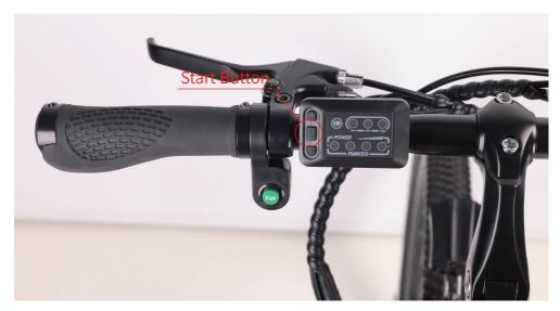
3.**Turn on the headlight** if needed or desired. Once the controller is on, press "\[ \times \]" button to turn the headlight on. Press it again to turn the headlight off.
