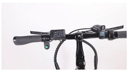
4.Tilt the LCD display to the optimal position and tighten the bolts.
