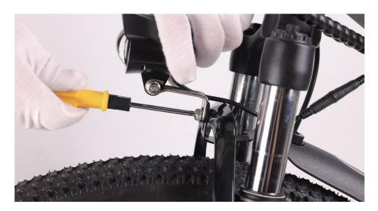
4.Center the headlight and adjust the angle slightly downwards to illuminate the road ahead and not blind oncoming traffic. Use the supplied Phillips-head screwdriver to loosen the headlight angle adjustment bolt, tilt the headlight to the optimal position, and then tighten in place securely.
