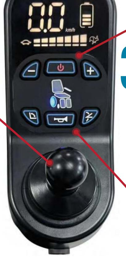
Immediately press the horn button. The controller will beep, and the chair will begin the unfolding process. Once the automatic unfolding process is complete, the controller will emit a final alarm, and it will automatically enter drive mode. The wheel indicator light will illuminate.
