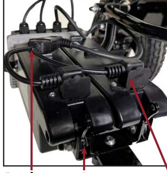
**Battery** Dual Locking Battery **Mechanism** Connector
