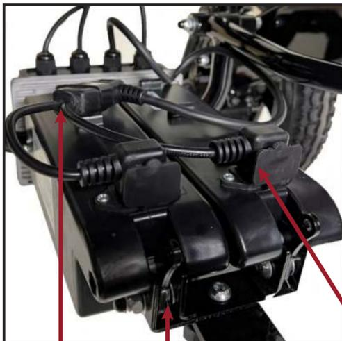
Dual Battery Connector      Battery Locking Mechanism
