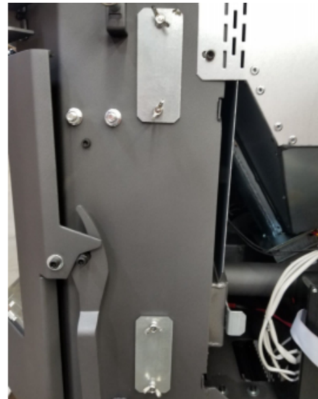
Figure 23: Exhaust Chamber Cover Plates. Air Intake side
