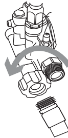
Figure 2-11. Connect Water Supply Hose
