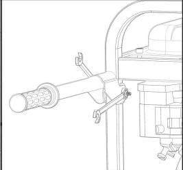
6. Repeat steps 3, 4, and 5 on the parallel frame leg, using the remaining handle, bolt, nut, and washers.
