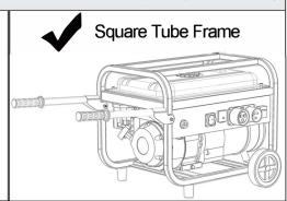
1A. If generator has existing handles, loosen and remove handle bolts and handles (If handle bolts or handle bolt holes exist in vertical frame, skip to step 3).
