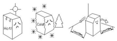
The distance between the air outlets and the wall should be over 20 cm. Besides, keep good ventilation and ensure the machine is dry and clean. The position to place the ice maker must be far away from the heat source, such as a bake oven, electric cooker, etc.
