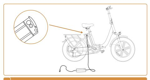
1 Make sure the power is turned off and check the connection of the charging cable and power adapter
