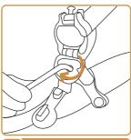
Tighten the bolt into the head tube.
