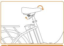
Insert the battery key, Turn it to the unlocked position.
