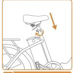
3 Loosen the seat clamp and adjust the seat to an appropriate angle.
