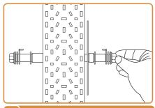
lnsert the front axle into the wheel hub from one side and install the bushings, spacers, safety hooks, spacers, and nuts on the axle in sequence from both sides
