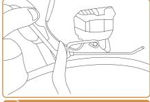
Put the fender through the front fork. Reinstall the bolts, washers and nuts (in this order). Reinstall the lower fender screws.
