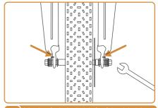
Adjust the safety hook to hook the front fork, and check that the front fork dropouts, safety hooks, spacers, and nuts are in sequence from the wheel hub to the outside. After ensuring the correct order, tighten the nuts with wrenches
