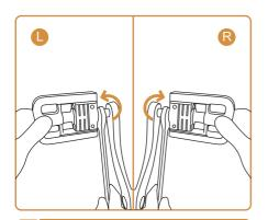
Fully tighten the pedals with a pedal wrench or open-end wrench.
