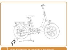
Plug the charger AC plug into a wall socket (100V-240V), and plug the DC connector into the electric bike's charging port.
