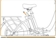
The battery is installed into the frame and can be taken out from the folded position of the frame.
