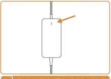
After charging for about 7 hours, the indicator light of the power adapter will change from red to green. Disconnect all cables when charging is complete.
