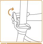
After tightening the bolt, Lift the stem and close the folding lock firmly.
