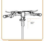
Adjust the handlebar to make it perpendicular to the front tire.
