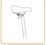
Close the seatpost clamp and make sure the seatpost is held in place. Don't adjust the seat too high (keep the safety line mark lower than the top of the seat tube).
