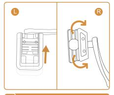
Push the pedal inward to fold the pedals up or down.
