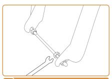
After taking out the front wheel, remove the front fork from the fork mount
