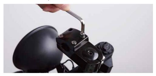
2.Place the handlebar on the stem correctly. Trace the front brake cable directly up from the front brake caliper to the left handlebar and ensure the cables and wires are not twisted. **Notice:** The horn is on the left hand side and the gear shift is on the right.
