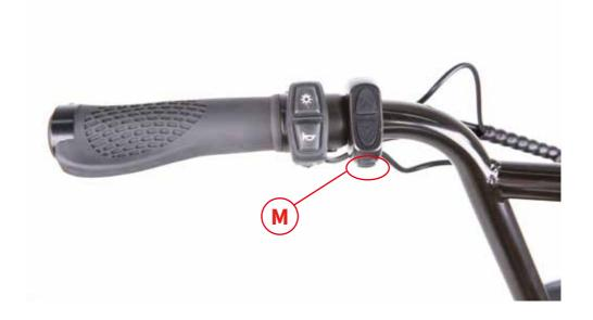
3.**Select the desired level of pedal assistance**—Select the level from 0-5 by pressing "+" and "-". Level 1 corresponds to the lowest level of pedal assistance, and level 5 corresponds to the highest level of pedal assistance. Level 0 indicates pedal assistance is inactive. Start in PAS level 0 or 1 and adjust from there.
