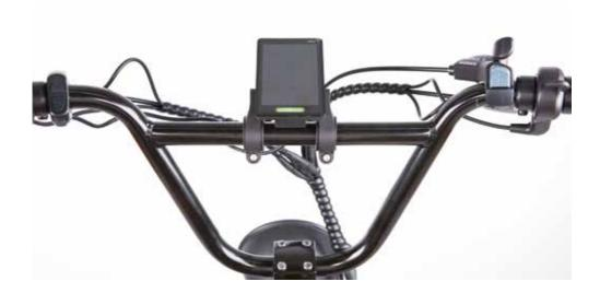
4.Tilt the LCD display to the optimal position and tighten the bolts.
