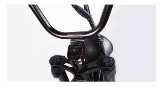
3. Center the handlebar and tighten the bolts on stem faceplate evenly.
