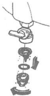
Fuel Filter Element Removal
