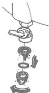
Fuel Filter Element Removal
