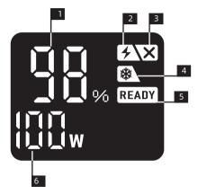
**1. Battery capacity percentage**: battery percentage of charge/discharge
