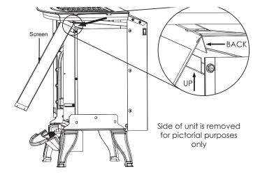
5. Remove the log box from inside the unit. Lift the unit off the pallet. NOTE: Make sure to lift the unit up high enough to clear the upright supports the unit is sitting on.
