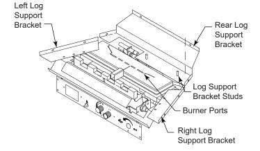
To install the back log (#1), position on rear log support bracket and then press down over studs.
