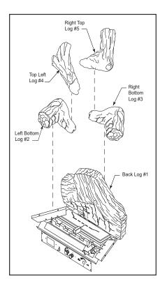
2. Install left bottom log (#2) on left log support bracket in front of back log.
