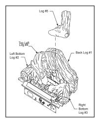
5. Install top right log (#5) on top of right bottom log.
