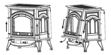
4. Remove the two screws located at the bottom of the screen as shown. Lift up and back on the screen to remove.
