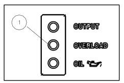
The overload indicator light ① comes on when the total wattage exceeds the generators capability. If that happens, proceed as follows:
