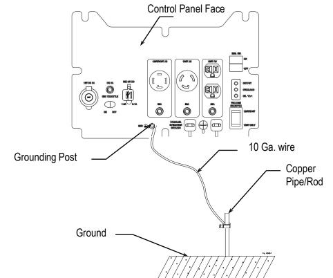
If a licensed electrician installs the generator with a connection to your building's electrical circuit for use as a back-up power system, grounding may alternatively be completed through the building's grounding system. Ask your electrician. If the generator is not grounded through your building's electrical system, follow the procedure above.
