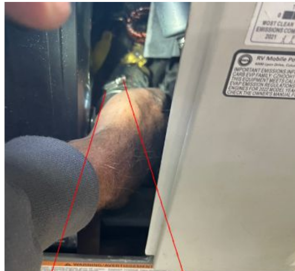
Worm clamp that secures fuel pump to mounting bracket
