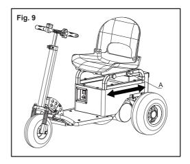
\* Tow bar connector height adjustment (See Fig. 10)
