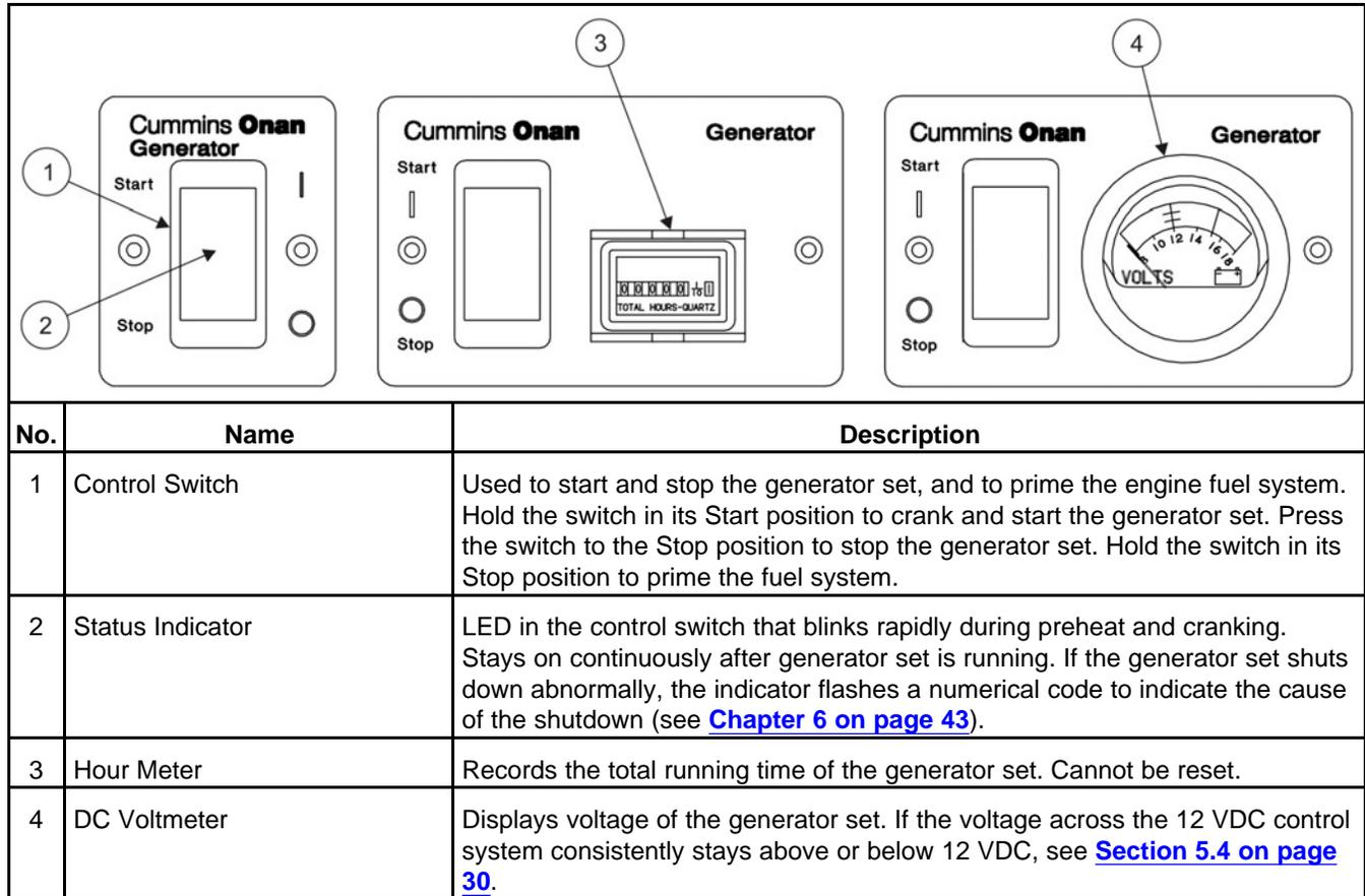
FIGURE 4. REMOTE CONTROL PANELS
