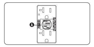
To ensure proper operation of the GFCI duplex, perform this test monthly:
