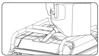
Screw on the fuel cap and wipe away any spilled fuel.
