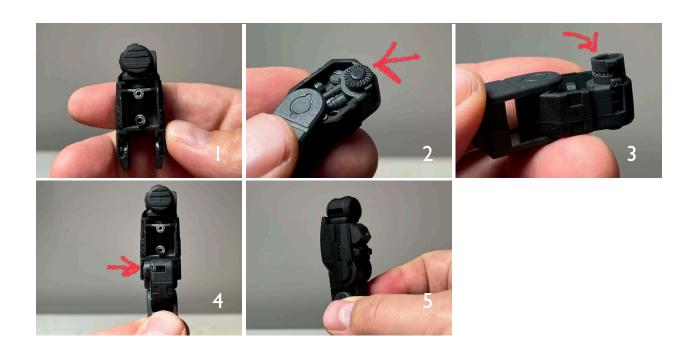
\*\*\*Attach the hip joint to the front of the upper leg. Add the spring and half the clicker joint to the knee. place the other half of the clicker joint on top of the first. Squeeze together and insert in the front upper leg. Add the back half and screw together.\*\*\*
