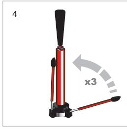
When folding the legs back up, hold onto the red aluminum pipe with one hand while folding the leg with another. Be careful to keep your fingers away from the pinch-points on the base when folding the legs back. Pull up on the three self-locking legs to unlock them and fold them up along the pipe.
