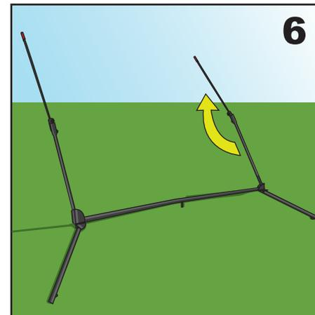
6. Fully extend the fiberglass top half of the left pole. The arms should be slanted in the same direction, as shown above.
