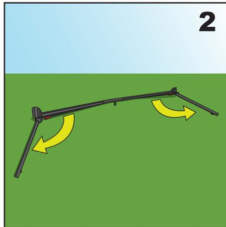
2. Unfold the legs, making sure that the locking button is fully extended.
