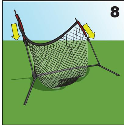
8. Slide the red sleeves completely over the fiberglass poles. Use ties to attach the bases of the red sleeves through the holes on the bases of the fiberglass arms.
