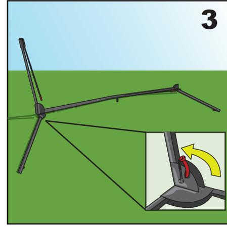
3. Bring up the left arm. Lock it into place using the base pin. Make sure the pin is fully inserted into the base.
