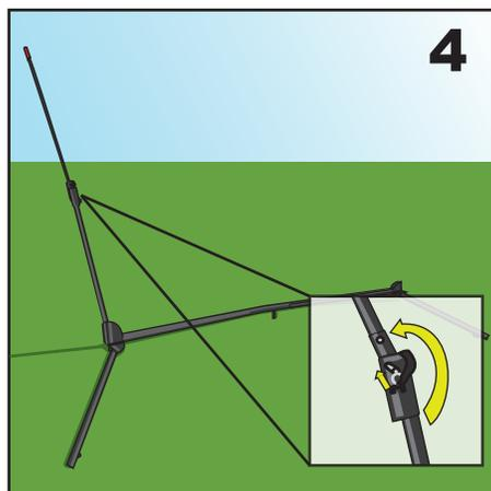
4. On the left arm, fully extended the fiberglass top half of the arm. Lock into place with the cotter pin.
