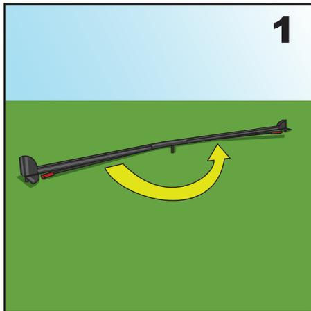
1. Unfold the frame's middle cross beam. The frame will lay flat on a rubber base.
