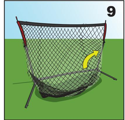
9. Pull the left arm fully upright and make sure that the base pin is fully inserted into the slot.
