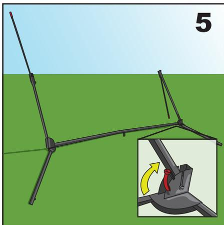
5. Bring up the right arm, but do not extend it all the way up. Rest the base pin on the groove that is half way up the bottom base plate.
