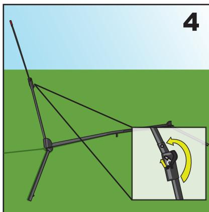
**4.** On the left arm, fully extend the fiberglass top half of the arm. Lock into place with the cotter pin.
