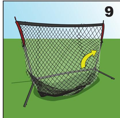
9. Pull the left arm fully upright and make sure that the base pin is fully inserted into the slot.
