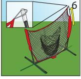
Gripping the assembled fiberglass pole, slide the net's sleeve up the pole and loop the white rope onto the metal knob on top.
