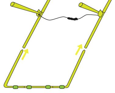
Attach the lower front assembly to the middle bars to complete the front of the rebounder.
