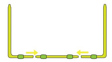
Attach the two lower legs with silicone traction pads to the remaining bottom crossbar to make the rear support assembly.
