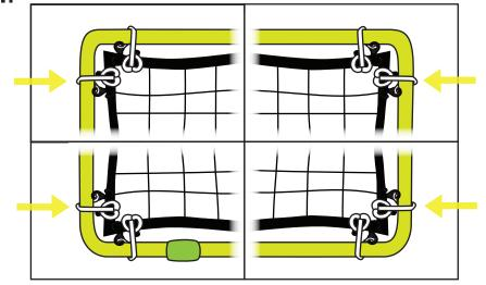
Stretch the netting side-to-side by hooking the 4 remaining corner bungees around the side bars.
