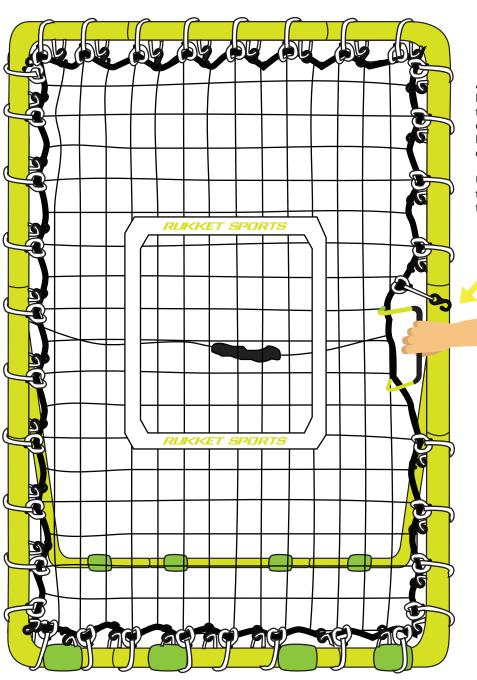
Alternate adding the remaining bungees between the top, bottom, left and right to ensure that the netting is stretched evenly. We suggest using all of the bungees, spaced 3 to 4 squares apart, to create maximum rebounding action.
