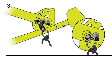
Screw the plunger bolts into the welded on nut and tighten down. Pull the cord to disengage the plunger and release it to allow the plunger to engage one of the holes. Set both of the rear support middle bars at the same setting so that they are both at the same angle.
