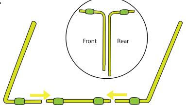
Attach the front legs with the silicone traction pads to one of the bottom crossbars (both bottom crossbars have silicone traction pads).
