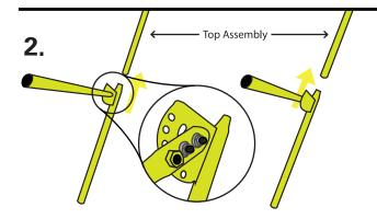
Attach the middle bars with angle-adjustment plates to the top assembly. The adjustment plates should be near the top of the rebounder and the support bar that moves along the plate should be on the inside of the rebounder.
