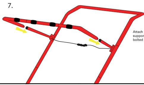
Attach the rear support assembly to the rear support middle bars. When the frame is securely bolted together, stand it up.
