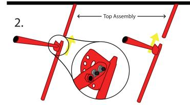
Attach the middle bars with angle-adjustment plates to the top assembly. The adjustment plates should be near the top of the rebounder and the support bar that moves along the plate should be on the inside of the rebounder.
