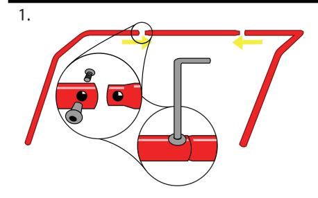
Join both top, side bars to the top crossbar. The fatter, circular receiving nut goes into the round hole and the outside-threaded bolt with the squared neck under the head goes into the square hole. Once you've threaded the bolt into the nut correctly, seat the square bolt neck into the square cut-out in order to tighten the nut with the hex key.
