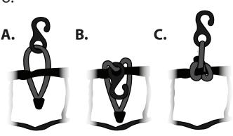
Attach the bungees to the thick woven edge of the netting by using a girth hitch. Hitch 2 bungees in each of the 4 corners of the netting. These 8 bungees will stretch the netting up-and-down and side-to-side. The bungees should not cross each other.
