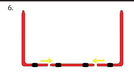
Attach the two straight lower legs with silicone traction pads to the remaining bottom crossbar to make the rear support assembly.
