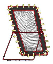
The bungies should be placed between the net's attaching hooks. Two bungies should be used on each corner and two bungies should be used on each side of of the pivot joint. More bungies are included so that you can customize how powerful you want
