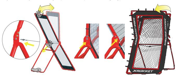
To adjust the Rebounder's over-all angle, simply push both adjustment buttons on the **Rear Telescoping Supports** and select the desired angle.
