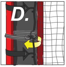
D. Hook the plastic onto the net's thick woven edge next to where the **Bungie** is hitched.
