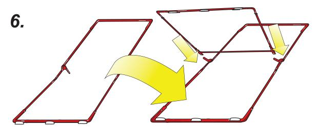
6. Attach the assembled rear support structure to the Pivot Joint by the slightly shorter tube on the U-Curve. The silicone pads on the Rear Base should be facing slightly inward so that they come in contact with the ground when the Rebounder is
