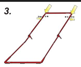
3. Attach the Top Cross Bar to the long tube of the Pivot Joints.
