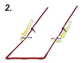
2. Attach the **Pivot Joint** to the **Front Supports.** Attach the slightly longer tube on the U-curve to each support.
