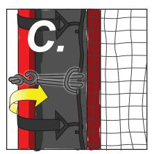
C. Pass the plastic hook in front of and around the metal frame.
