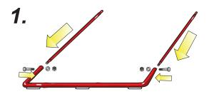
1. Attach the two **Front Supports** to the **Front Base** so that the silicone pads are angled slightly down when laying flat on the ground.
