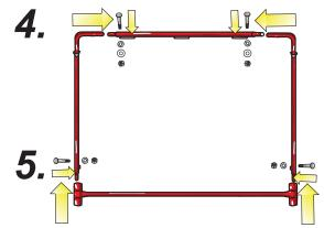
4. Attach the Rear Base to the two Rear Telescoping Supports so that the Adjusting Buttons face inside. Use the two plastic washers to ensure that the carriage bolts tighten completely.
