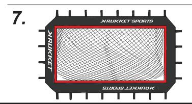
7. Stand the Rebounder up and make sure that the frame is assembled correctly before attaching the net.
