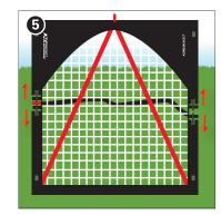
Run the remaining four fiberglass poles through the net's side sleeves and attach them to the black corner joints. Make sure the fiberglass poles are seated all the way into the corner joints.
