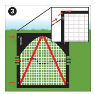
Run two of the poles through the top front and bottom rear sleeves by using the assembly windows.
