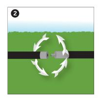
Assemble all the fiberglass poles by screwing them tightly together.
