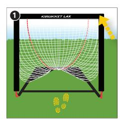
Fold your lacrosse goal by pushing the top front right corner diagonally down and back toward the rear bottom left corner. The net will then lay flat on the ground.
