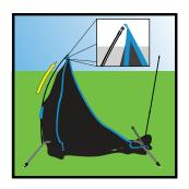
5. Gripping the assembled fiberglass pole, slide the net's sleeve up the pole and loop the white rope onto the metal knob on top.
