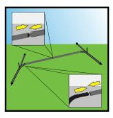
Join the two slightly bent pipes together. Then attach both end legs
