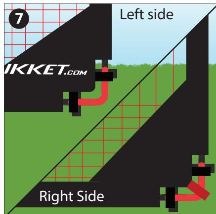
Wrap and velcro together the black straps around the red corner joints to secure the net.
