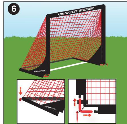
Connect the two fiberglass poles to each other with the red corner joints that have stakes attached. These red corner joints will remain exposed. We suggest attaching the red corner joints to the base poles first, and then lifting the front of the goal up vertically so as to slide the front poles down into the corner joints. Make sure the fiberglass poles are seated all the way into the corner joints.
