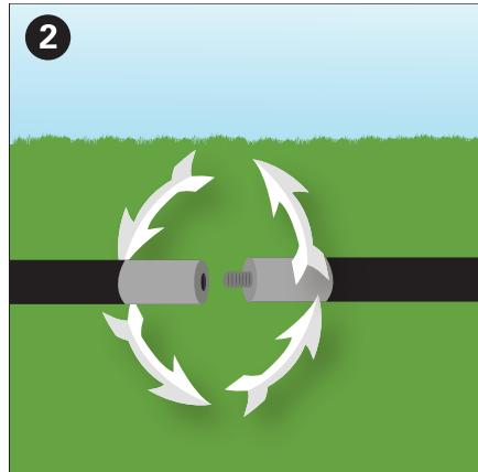
Assemble the fiberglass poles. The four four-foot poles connect to make two 8-foot crossbars. The eight 3-foot poles connect to make four 6-foot side bars.
