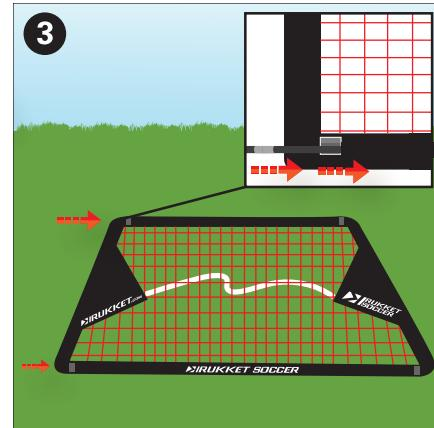
Run the two 8-foot crossbars through the longest sleeves (the top front and the rear bottom sleeves) using the assembly windows.
