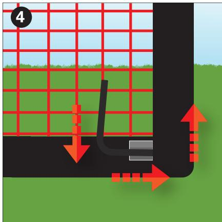
Attach the four black corner joints to the two crossbars using the assembly windows so that they give structural form to the net's four corners. Make sure that the crossbars are seated all the way into the corner joints.
