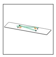
3. Take the second glow stick and slide it diagonally into the other two clips. This stick will sit on top of the stick attached in Step #2.
