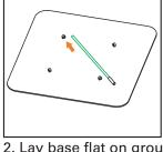
2. Lay base flat on ground with clips facing up. Take one of the connector tubes and attach it to one end of the stick. Slide the stick diagonally into one clip.
