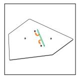
2. Lay the base flat on the ground with the clips facing up. Take one of the sticks and slide it diagonally into the clips.
