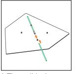
3. Then, slide the second stick diagonally through the second clip and attach it to the connector tube.
