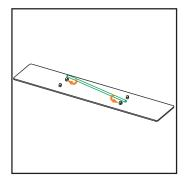
2. Place the plate with the clips facing up. Take one of the glow sticks and slide it diagonally into the clips.
