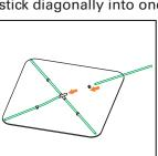
5. Then slide the fourth stick diagonally through the final clip and attach the connector tube.
