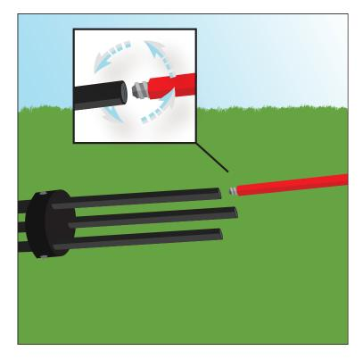
Before using your Rukket Ball Caddy, you will need to attach the legs to the upper portion. Screw the red legs into black pipes and tighten all the way.
